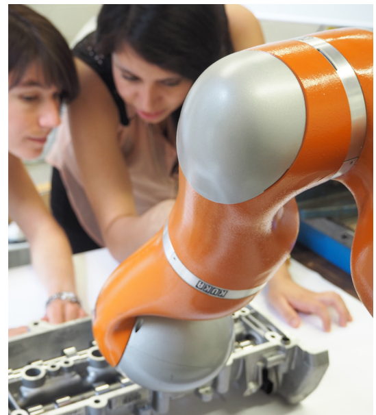
_Figure 1: comprehensive challenge: Robotic Grinding, an interplay of free form following and grinding process
